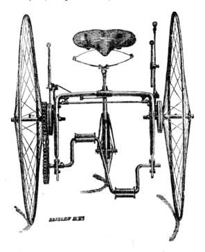
Fitted with a new adjustable band brake, adjustable handles, horn handles and plated hubs, handle brackets, seat and steering rod, new seat-rod adjustment (exceedingly simple), new triangular roller bearing pedals, &c.; ordinary width, 3 feet 3 inches, can be made narrower to order; by unscrewing the foot-rest or cap-nut the side wheel can be taken off, when the machine will pass through a doorway 2 feet 6 inches wide—a very great desideratum.
