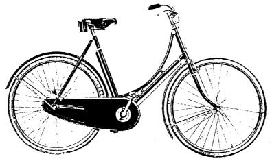
The Lady's fittings are designed to take 28 in, wheels, with clearance for 158 in, tyres a frame very taking in appearance, the lines of which have been very carefully considered.
