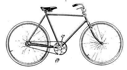
The Light Roadster machine, illustrated above, is built from "G" pattern fittings, and has necessary clearance for roadster tyres.
